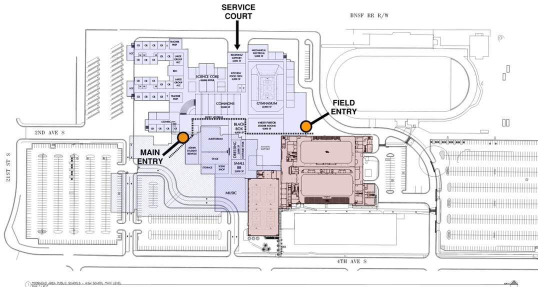
Workshop #2 JUNE 2020 – Reorient wings and relocate service to N side
