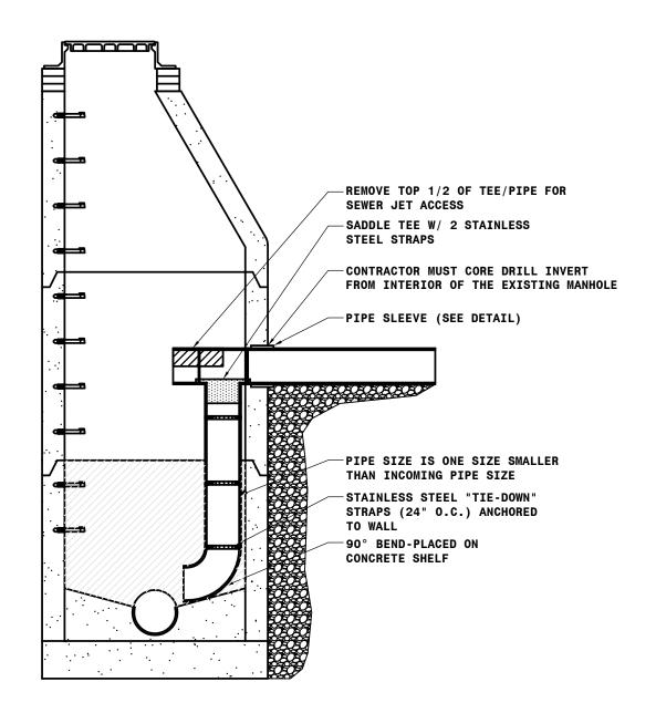
5 SANITARY SEWER MANHOLE (INTERIOR DROP CONNECTION) DETAIL (BY 33) 08.0 NOT-TO-SCALE
